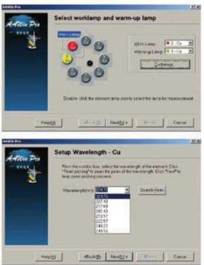
Lamp turret setup, operating and warm-up currents, along with the desired analytical wavelength are easily selected in the configuration.
